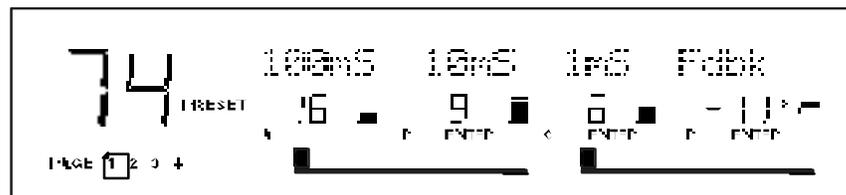
The actual delay time can be derived by adding these three parameters together. For example, in the display above, the Delay Time value equals 1696 ms.
