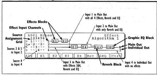
The Value dial (RI) selects the effect algorithm to be used. There are four different algorithms available, and the arrangement of the effects blocks varies depending upon the algorithm chosen.
