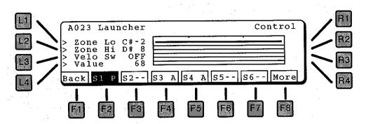
This screen has parameters for key and velocity range. Using these parameters, a sound can be limited to play in only a certain range of the keyboard, or only when a key is played hard or soft. By creating several sources, for example, one that plays on soft notes only and another that plays on hard notes only, a sound can be created with more lifelike variation.
