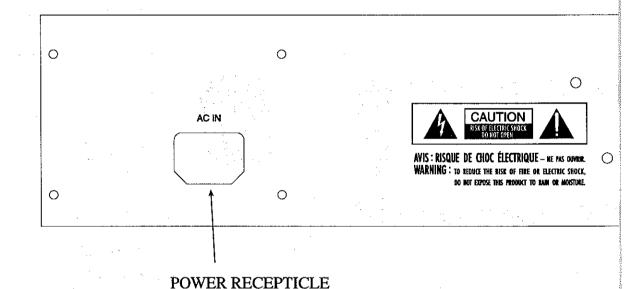
Apply power here (120 Volts AC / 60Hz)
