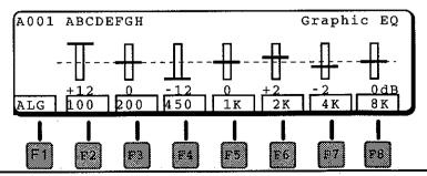
Use the F2 through F8 keys to select an EQ band, and the Value dial to change the amount. The slider will change to visually indicate the setting, the number underneath shows the exact amount.
