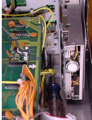
Only 2 screws remain holding your DSM-1 disk drive in place. They are on the upper flange of the drive bracket. They are relatively easy to remove. As you can see in the photo to the right, I elected to use some hemostats to capture these screws as they were removed so as not to drop them into an area where I might have trouble retrieving them. Once you have these last two screws removed, the disk drive (still attached to the drive bracket) will be disconnected and ready to remove.
