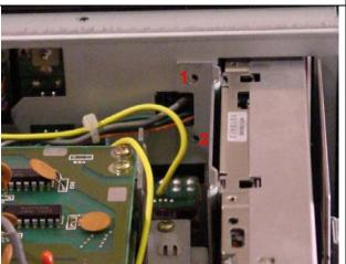
The disk drive and bracket remove as one assembly. Simply pull back on the drive until the front panel is cleared and then lift the drive up and out of the DSM-1.
