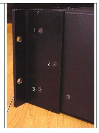
The next step is to remove the top cover of the DSM-1 There are 10 screws that hold the cover in place. You will find 2 on each side, 3 across the top near the front edge and 3 on the back. See the three photos detaining which screws to remove.
