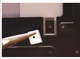
Flip the DSM-1 up on its side (with the disk drive side to the top). Remove the two screws from the bottom as shown in the photo to the right. These hold the drive bracket to the bottom.
