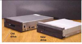
The new drive must be attached to the drive mounting bracket before it can be installed. Slide the bracket over the drive and attach using the same 4 screws that held the original drive to the bracket.
