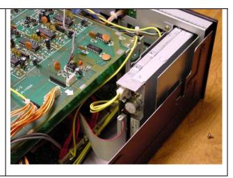
Here is what your new drive looks like from the front when the installation is complete. The trim fit is not perfect, but your DSM-1 is now working again. Connect the power and test the operation of your new disk drive. If everything works as it should, replace the top cover and secure with the 10 screws originally removed. Replace the 2 rack ears and fasten them with 3 screws each.
