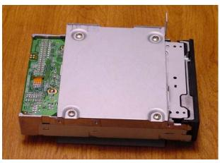
Your new drive mounted on the drive bracket should look like the photo below on the left. Notice that there is some additional space between the new drive and the side of the drive mounting bracket. Before you slip the new drive and bracket into place, insert the lower flange mounting screw through the hole in the lower flange as shown in the lower right photo. This is about the only way you can get that screw back into that tight spot. This worked great for me.
