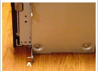
Carefully lower the new drive and bracket assembly into the DSM-1 and slide forward into position. Before pushing all the way forward, position your screwdriver to guide the lower flange screw into the hole in the front panel. This will be the first screw installed. It may be difficult to get started. So, be patient and turn your screwdriver in small increments each time. Do not tighten the screw 100%. You will install all 5 of the drive bracket mounting screws and then tighten them all.
