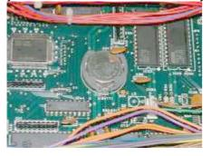
7. To remove the battery push it carefully towards the back of the holder at which point the battery should come lift out quite easily.
