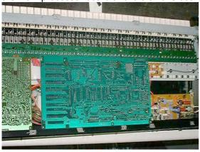
3. You will see two cables emanating from the right hand edge of this board. One of these will run to a connector just below the key frame, which is in turn attached to a small PCB board. Remove this connector.
