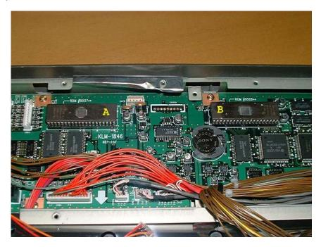
These will normally be situated in sockets, which are in turn soldered into the board. If you Remove the paper label from one IC you should find a small window which denotes that it is an EEPROM and therefore re-programmable. (See C below)
