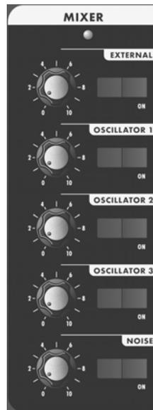
The Mixer combines the main sound sources of the Voyager. It's the place to start when creating a new sound from scratch, or figuring out how a sound is put together. All the sound sources can be turned on or off, and their levels can be adjusted. The sound sources available are:
