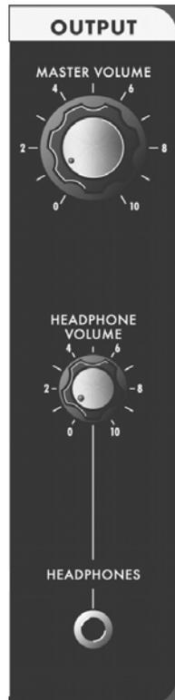
The Voyager has two audio outputs. There is a VCA for each output, which allows for stereo effects such as Panning or the Dual lowpass filtering. The main control for the Volume is the Master Volume Control. The Volume Envelope modulates the output VCAs. When only one output is desired, the two output VCAs are mixed to the left output.
