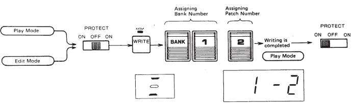
\*If the Protect Switch has been set to ON, no writing is done and the Display will show "Protect" on, right after assigning Patch Number.
