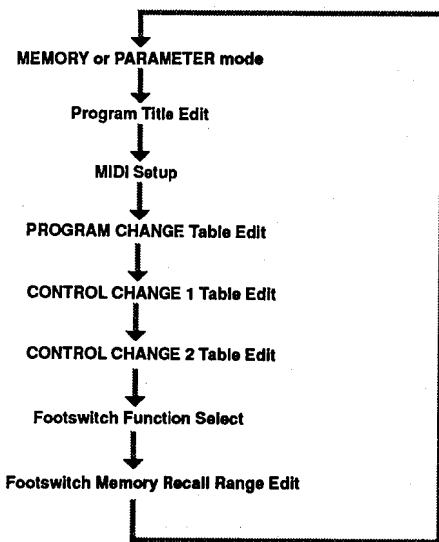
The mode that was active before the UTILITY key was pressed (MEMORY or PARAM) is selected following the last function on the utility list. The UTILITY mode can also be exited by pressing several times or holding (about one second) the UTILITY button until the UTILITY key indicator goes out.
