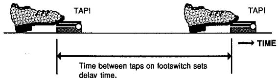
**CAUTION:** If either the L-DLY or R-DLY parameter is set to its maximum or minimum value, the TAP TEMPO DELAY function cannot be used to create longer or shorter delays.
