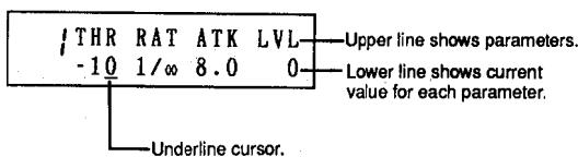
The PARAM mode can not be directly selected from the UTILITY mode by pressing the PARAM key. The UTILITY mode must first be exited by pressing several times or holding (about one second) the UTILITY key until the UTILITY key indicator goes out.
