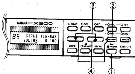
Once the MIDI controllers you wish to use have been selected using the Control Change 1 Table Edit and Control Change 2 Table Edit functions described above, you can then assign the controllers to the specific FX500 effect parameters. Control assignment is carried out in the PARAM mode.
