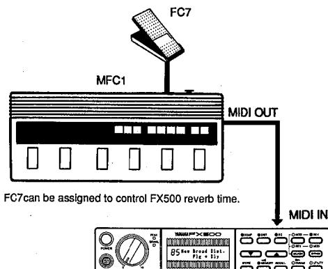
FC7 can be assigned to control FX500 reverb time.
